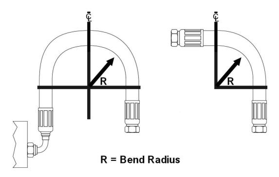
The minimum bend radius is measured from the inside of the hose to the centerline of the bend.
