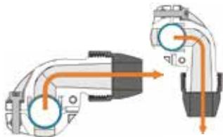
Quickdrop design safeguards leaktight and condensate free droplines
